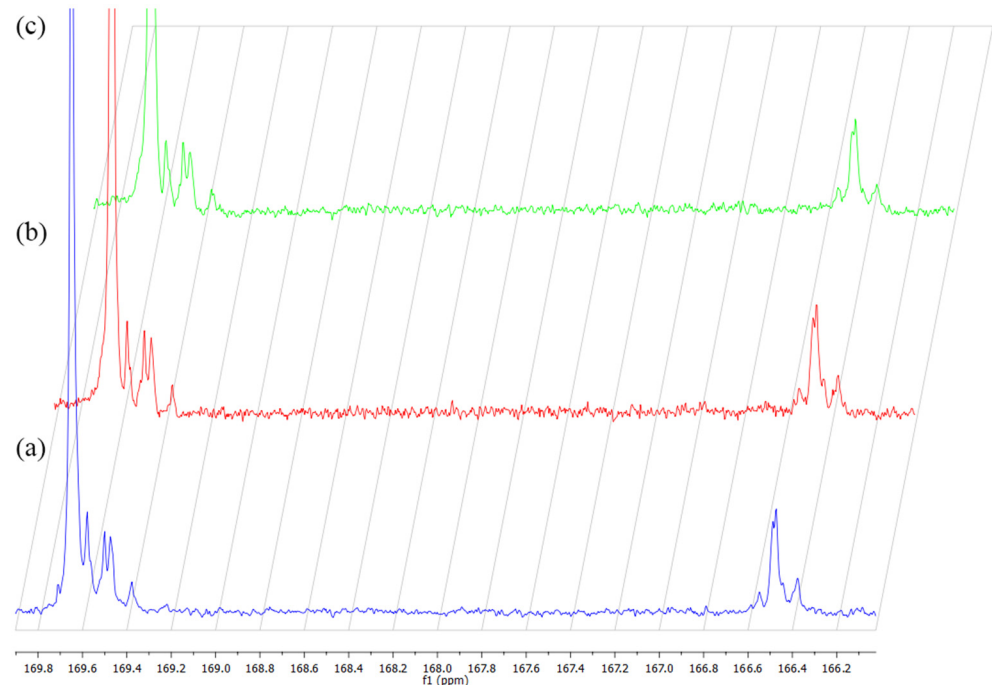
Figure 1. The influence of ionizing radiation on ^{13}C NMR spectra of PLGA non-irr (a), irr- \gamma (b) and irr- e^- (c).
