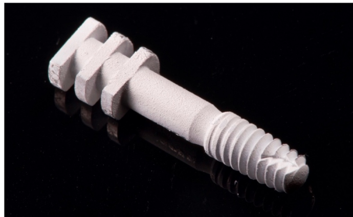
Figure 2. Implant model with an attached closed tray impression transfer prepared for scanning.
