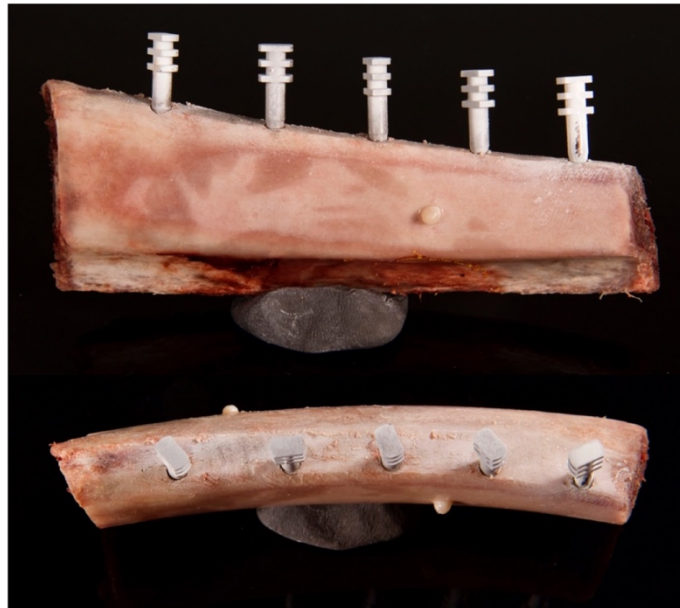
Figure 1. Bone model containing five implants with attached closed tray impression transfers coated with scan spray. Implants were placed with different bone margin thickness. X-ray markers made of dental composite were attached to the bone model surfaces.
