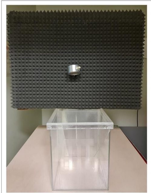
FIGURE 4 | The photograph of the VOC-NCE located in the behavioral recording room (the frontal view). For clarity, cables have been unplugged from the microphones, and the covering grid was removed.
